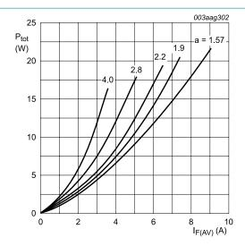
a = form factor =  $I_{F(RMS)}/I_{F(AV)}$  $V_o$  = 0.987 V;  $R_s$  = 0.065  $\Omega$
