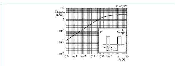
Fig. 4. Transient thermal impedance from junction to mounting base as a function of pulse width
