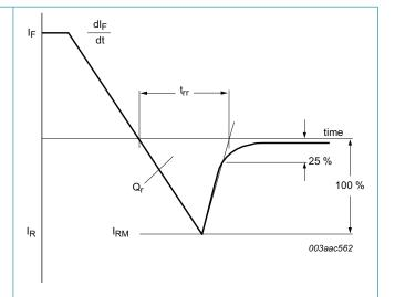
Fig. 6. Reverse recovery definitions; ramp recovery
