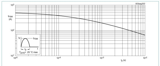
Fig. 3. Non-repetitive peak forward current as a function of pulse width; sinusoidal waveform; maximum values
