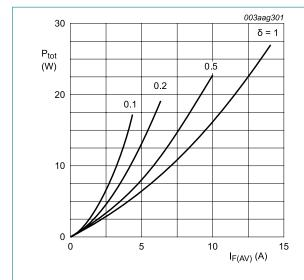
$\begin{aligned} I_{F(AV)} &= I_{F(RMS)} \times \sqrt{\delta} \\ V_o &= 0.987 \text{ V}; \text{ R}_s = 0.065 \text{ }\Omega \end{aligned}$
