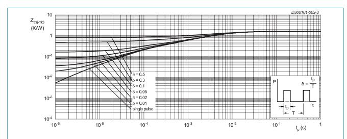
Fig. 3. Transient thermal impedance from junction to mounting base as a function of pulse duration; maximum values
