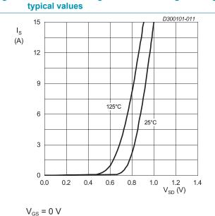
Fig 11. Source current as a function of source-drain voltage; typical values
