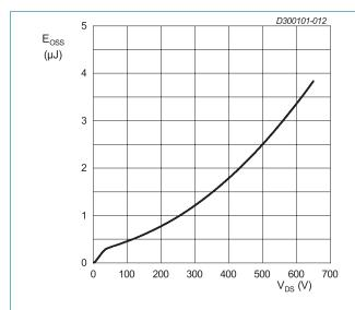
Fig. 12. Output capacitance stored energy as a function of drain-source voltage
