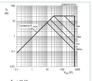
$T_{mb}$  = 25 °C Fig. 13. Safe operating area
