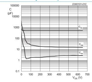
V<sub>GS</sub> = 0 V; f = 1 MHz Fig 10. Capacitances as a function of drain-source voltage; typical values
