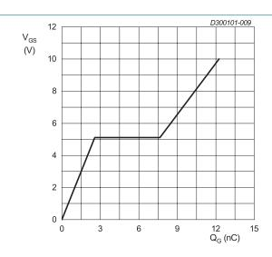
$I_D = 3.5 \text{ A}$ ;  $V_{DS} = 400 \text{ V}$ Fig. 9. Gate-source voltage as a function of gate charge;
