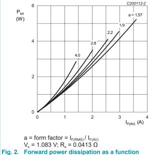
of average forward current; sinusoidal waveform; maximum values
