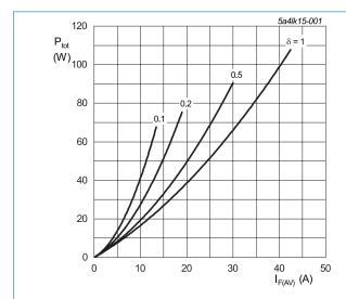
$I_{F(AV)} = I_{F(RMS)} \times \sqrt{\delta}$   $V_o = 1.383 \text{ V; } R_s = 0.0273 \Omega$
