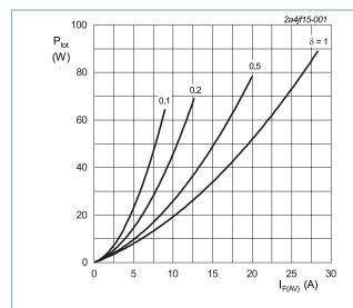
$$\begin{split} I_{F(AV)} &= I_{F(RMS)} \times \sqrt{\delta} \\ V_o &= 1.268 \text{ V; } R_s = 0.0662 \text{ } \Omega \end{split}$$
