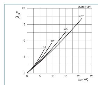
$\begin{aligned} &I_{\text{F(AV)}} = I_{\text{F(RMS)}} \times \sqrt{\delta} \\ &V_{\text{o}} = 0.656 \text{ V; } R_{\text{s}} = 0.0066 \text{ } \Omega \end{aligned}$
