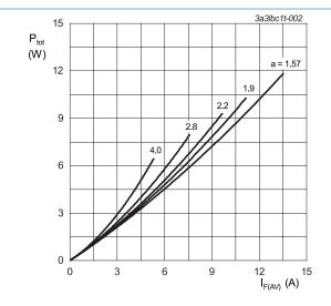
a = form factor =  $I_{F(RMS)}$  /  $I_{F(AV)}$ V<sub>o</sub> = 0.656 V;  $R_s$  = 0.0066  $\Omega$
