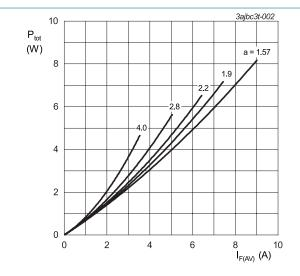
a = form factor =  $I_{F(RMS)} / I_{F(AV)}$  $V_o$  = 0.644 V;  $R_s$  = 0.0119  $\Omega$
