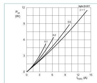
$I_{F(AV)} = I_{F(RMS)} \times \sqrt{\delta}$   $V_0 = 0.644 \text{ V}; R_s = 0.0119 \Omega$ in 1. Forward power dissipation as
