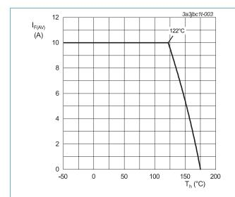
Fig. 3. Average forward current as a function of heatsink temperature; maximum values; per diode
