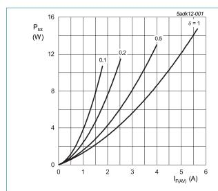
$\begin{aligned} I_{F(AV)} &= I_{F(RMS)} \times \sqrt{\delta} \\ V_o &= 1.044 \text{ V; } R_s = 0.2758 \text{ }\Omega \end{aligned}$
