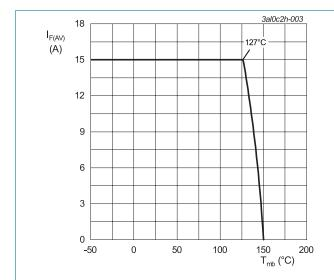
Fig. 3. Average forward current as a function of mounting base temperature; maximum values; per diode
