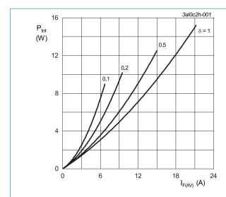
$$\begin{split} & |_{\text{F(AV)}} = |_{\text{F(RMS)}} \times \sqrt{\delta} \\ & |_{\text{O}} = 0.430 \text{ V; R}_{\text{s}} = 0.0135 \text{ }\Omega \\ & \text{Fig. 1. Forward power dissipation as a function of average forward current; square waveform;} \end{split}$$
