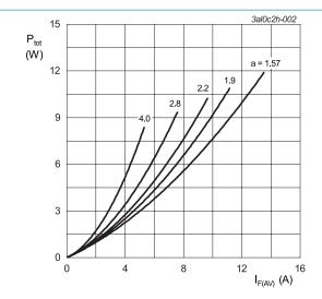
a = form factor =  $I_{F(RMS)}$  /  $I_{F(AV)}$  V<sub>o</sub> = 0.430 V;  $R_s$  = 0.0135  $\Omega$
