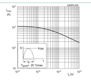
Fig. 4. Non-repetitive peak forward current as a function of pulse width; sinusoidal waveform; maximum values; per diode
