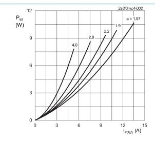
a = form factor =  $I_{F(RMS)}$  /  $I_{F(AV)}$ V<sub>o</sub> = 0.349 V; R<sub>s</sub> = 0.0132  $\Omega$
