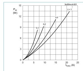
$I_{F(AV)} = I_{F(RMS)} \times \sqrt{\delta}$  $V_o = 0.349 \text{ V}; \text{ R}_s = 0.0132 \Omega$
