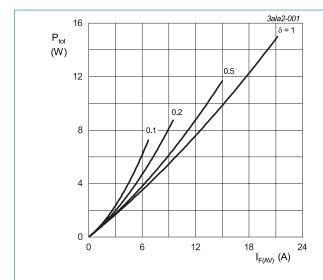
$I_{F(AV)} = I_{F(RMS)} \times \sqrt{\delta}$  $V_o = 0.534 \text{ V}; R_s = 0.0082 \Omega$
