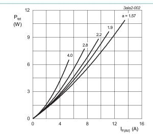
a = form factor =  $I_{F(RMS)}$  /  $I_{F(AV)}$ V<sub>o</sub> = 0.534 V; R<sub>s</sub> = 0.0082  $\Omega$
