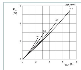
$I_{F(AV)} = I_{F(RMS)} \times \sqrt{\delta}$ V<sub>o</sub> = 0.651 V; R<sub>s</sub> = 0.0177 Ω
