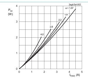
a = form factor =  $I_{F(RMS)}$  /  $I_{F(AV)}$  V<sub>o</sub> = 0.651 V;  $R_s$  = 0.0177  $\Omega$
