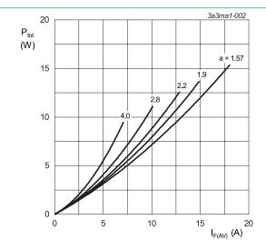
a = form factor =  $I_{F(RMS)}$  /  $I_{F(AV)}$ V<sub>o</sub> = 0.541 V; R<sub>s</sub> = 0.0070  $\Omega$
