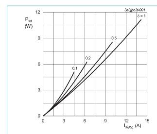
$I_{F(AV)} = I_{F(RMS)} \times \sqrt{\delta}$  $V_o = 0.625 \text{ V}; R_s = 0.0114 \Omega$
