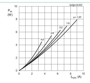
a = form factor =  $I_{F(RMS)}$  /  $I_{F(AV)}$ V<sub>o</sub> = 0.625 V; R<sub>s</sub> = 0.0114  $\Omega$
