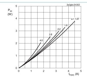
a = form factor =  $I_{F(RMS)}$  /  $I_{F(AV)}$  V<sub>o</sub> = 0.631 V;  $R_s$  = 0.0188  $\Omega$
