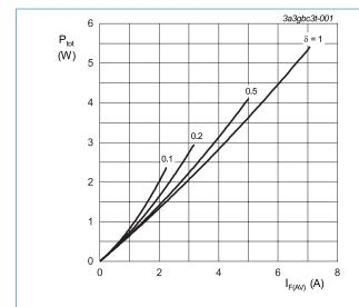
$\begin{aligned} & I_{F(AV)} = I_{F(RMS)} \times \sqrt{\delta} \\ & V_o = 0.631 \text{ V}; \text{ R}_s = 0.0188 \text{ }\Omega \end{aligned}$
