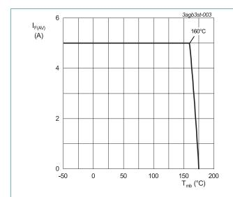
Fig. 3. Average forward current as a function of mounting base temperature; maximum values; per diode
