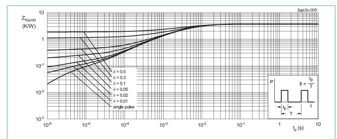
Fig. 5. Transient thermal impedance from junction to mounting base as a function of pulse duration; maximum values; per diode
