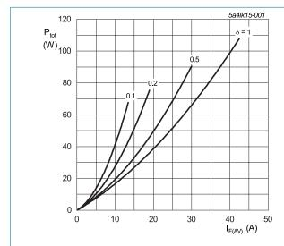
$$\begin{split} I_{F(AV)} &= I_{F(RMS)} \times \sqrt{\delta} \\ V_o &= 1.383 \text{ V; } R_s = 0.0273 \text{ } \Omega \end{split}$$
