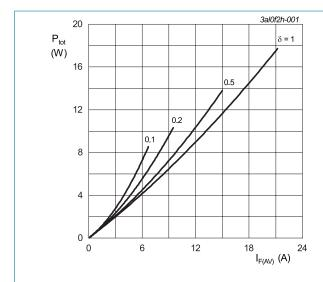
$I_{F(AV)} = I_{F(RMS)} \times \sqrt{\delta}$   $V_o = 0.633 \text{ V; } R_s = 0.0096 \Omega$
