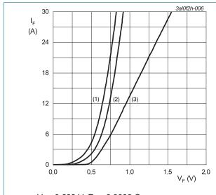
$V_o$  = 0.633 V;  $R_s$  = 0.0096  $\Omega$  (1)  $T_i$  = 150 °C; typical values
