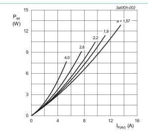
a = form factor =  $I_{F(RMS)}$  /  $I_{F(AV)}$  V<sub>o</sub> = 0.633 V; R<sub>s</sub> = 0.0096  $\Omega$
