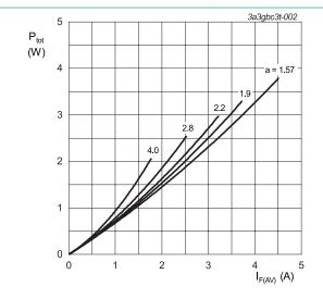
a = form factor =  $I_{F(RMS)} / I_{F(AV)}$  $V_o$  = 0.631 V;  $R_s$  = 0.0188  $\Omega$
