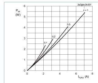
$$\begin{split} I_{F(AV)} &= I_{F(RMS)} \times \sqrt{\delta} \\ V_o &= 0.631 \text{ V; } R_s = 0.0188 \text{ } \Omega \end{split}$$
