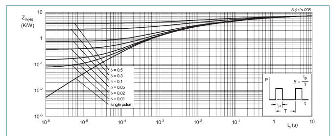
Fig. 5. Transient thermal impedance from junction to heatsink as a function of pulse duration; maximum values; per diode
