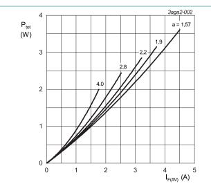
a = form factor =  $I_{F(RMS)} / I_{F(AV)}$  $V_o$  = 0.591 V;  $R_s$  = 0.0190  $\Omega$
