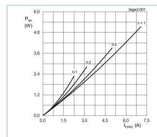
$I_{F(AV)} = I_{F(RMS)} \times \sqrt{\delta}$   $V_o = 0.591 \text{ V}; R_s = 0.0190 \Omega$ Fig. 1. Forward power dissipation a
