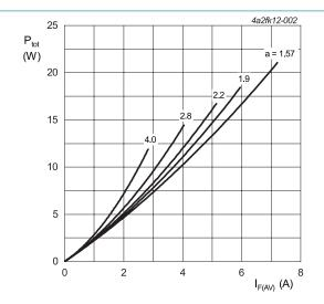
a = form factor =  $I_{F(RMS)}/I_{F(AV)}$ V<sub>o</sub> = 2.097 V; R<sub>s</sub> = 0.0464  $\Omega$
