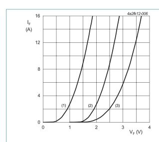
$V_o$  = 2.097 V;  $R_s$  = 0.0464 Ω (1)  $T_j$  = 150 °C; typical values (2)  $T_j$  = 150 °C; maximum values (3)  $T_j$  = 25 °C; maximum values
