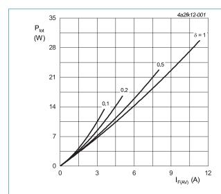
$\begin{aligned} I_{\text{F(AV)}} &= I_{\text{F(RMS)}} \times \sqrt{\delta} \\ V_{\text{o}} &= 2.097 \text{ V; } R_{\text{s}} = 0.0464 \text{ } \Omega \end{aligned}$
