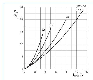
$I_{F(AV)} = I_{F(RMS)} \times \sqrt{\delta}$  $V_o = 1.395 \text{ V}; R_s = 0.1006 \Omega$
