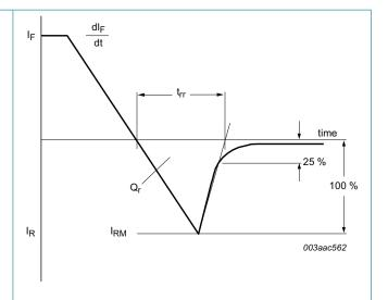
Fig. 6. Reverse recovery definitions; ramp recovery
