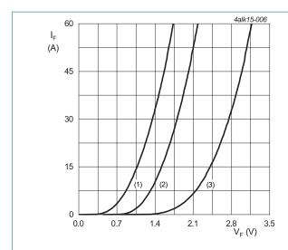
$V_o$  = 1.436 V;  $R_s$  = 0.0127 Ω (1)  $T_j$  = 150 °C; typical values (2)  $T_j$  = 150 °C; maximum values
