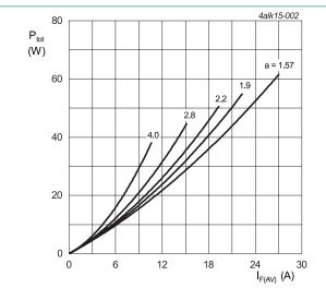
a = form factor =  $I_{F(RMS)}/I_{F(AV)}$ V<sub>o</sub> = 1.436 V; R<sub>s</sub> = 0.0127  $\Omega$
