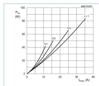
$I_{F(AV)} = I_{F(RMS)} \times \sqrt{\delta}$  $V_o = 1.436 \text{ V; R}_s = 0.0127 \Omega$
