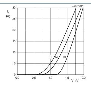
$\begin{array}{l} V_o=0.962~V;~R_s=0.0362~\Omega\\ (1)~T_j=150~^{\circ}C;~typical~values\\ (2)~T_j=150~^{\circ}C;~maximum~values\\ (3)~T_j=25~^{\circ}C;~maximum~values \end{array}$
