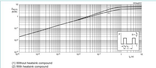
Fig. 6. Transient thermal impedance from junction to heatsink as a function of pulse duration
