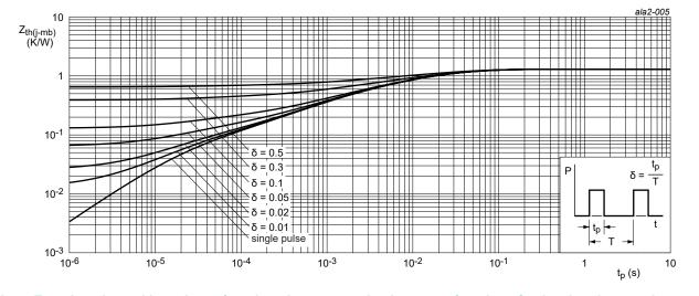
Fig. 5. Transient thermal impedance from junction to mounting base as a function of pulse duration; maximum values; per diode
