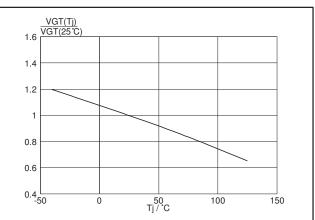
Fig.6. Normalised gate trigger voltage  $V_{GT}(T_i)/V_{GT}(25^{\circ}C)$ , versus junction temperature  $T_i$
