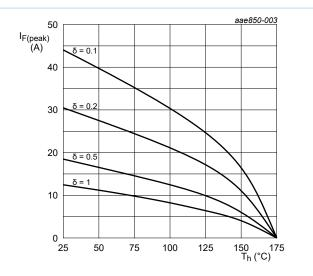
Fig. 4. Current derating as a function of heatsink temperature
