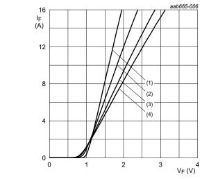
(1)  $T_j$  = 25 °C; typical values (2)  $T_j$  = 100 °C; typical values (3)  $T_j$  = 150 °C; typical values (4)  $T_j$  = 175 °C; typical values
