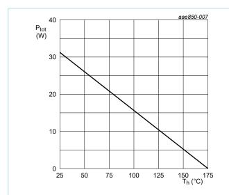
Fig. 3. Total power dissipation as a function of heatsink temperature
