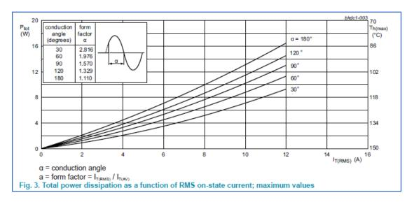
Fig. 9 Example of power dissipation graphic
