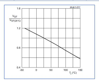
Fig. 26 Normalized V<sub>GT</sub> versus junction temperature
