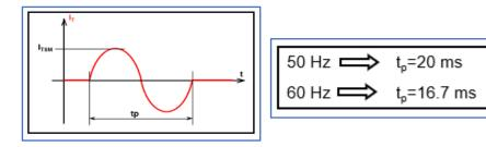
Fig. 10 Example of non-repetitive peak on state current rating
