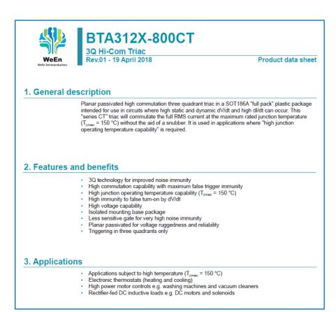
Fig. 1 Example of a datasheet product profile (BTA312X-800CT)
