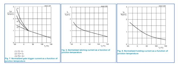
Fig. 23 I<sub>GT</sub>, I<sub>L</sub>, and I<sub>H</sub> temperature dependency graphics (BTA312-800CT)
