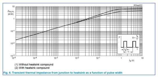
Fig. 19 Example of transient thermal impedance graphic
