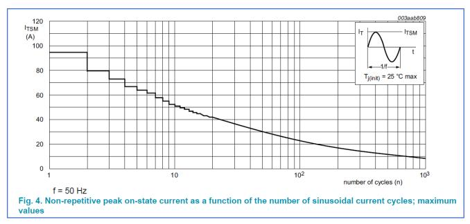
Fig. 12 Example of I<sub>TSM</sub> versus number of pulses
