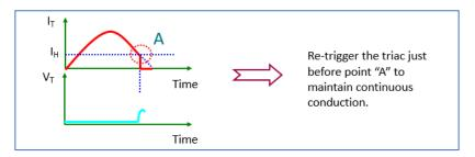
Fig. 25 Graphic showing interaction of I<sub>T</sub> and I<sub>H</sub>
