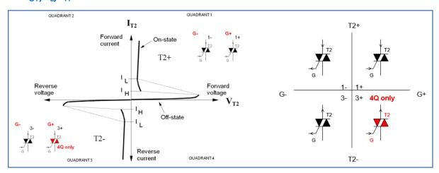
Fig. 20 Triac operating characteristic and triggering options
