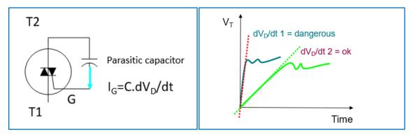
Fig. 31 dV<sub>D</sub>/dt illustration
