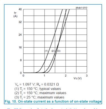
Fig. 27 Example of static characteristic V<sub>T</sub> and graphic
