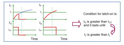
Fig. 24 Graphic showing interaction of I<sub>GT</sub> and I<sub>L</sub>
