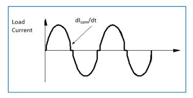
Fig. 33 dl<sub>com</sub>/dt illustration for a rectifier fed inductive load
