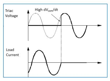
Fig. 34 dV<sub>com</sub>/dt illustration for an inductive load
