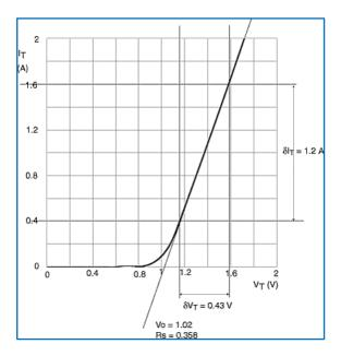
Fig. 28 Example graphic showing V<sub>0</sub> and R<sub>s</sub> derivation
