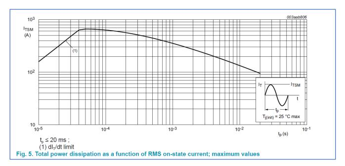
Fig. 11 Example of I<sub>TSM</sub> versus pulse width
