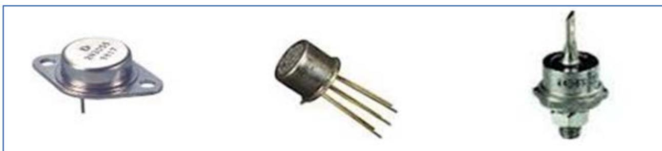
Fig.1 Examples TO3, TO5 and DO5 – older metal can power packages
