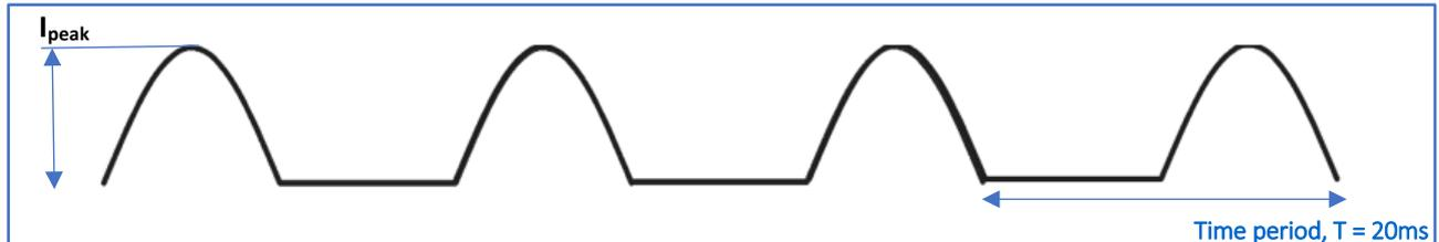
Fig. 2 Continuous current of 10ms half-sine waves
