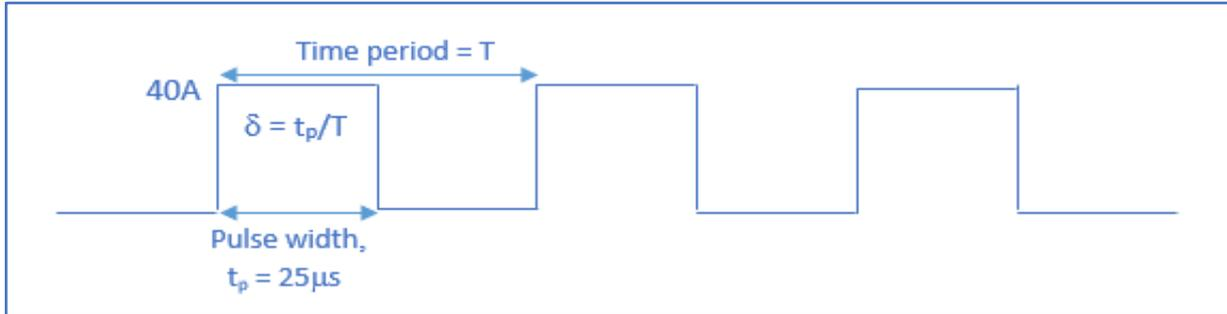
Fig.1 Peak current of 40A with  $\delta = 0.5$  and frequency =  $1/T$  Hz
