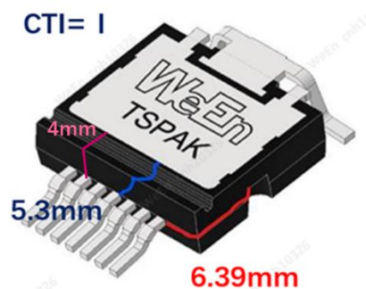
Fig. 15. Example of creepage distance between Drain and Source.
