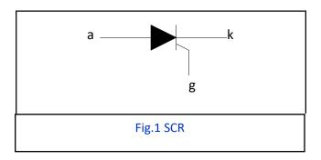
An SCR is a silicon-controlled rectifier (Fig. 1) where the unidirectional current flow from anode to cathode is initiated by a small signal current from gate to cathode. The SCR's operating characteristic is shown below in Fig. 2
