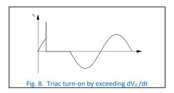
Rule 5. Where high  $dV_D/dt$  or  $dV_{COM}/dt$  are likely to cause a problem, fit an RC snubber across MT1 and MT2. Where high  $dI_{COM}/dt$  is likely to cause a problem, fit an inductor of a few mH in series with the load. Alternatively, use a Hi-Com triac.
