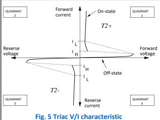
Where the gate is to be triggered by DC or unipolar pulses at zero-crossing of the load current, negative gate current is to be preferred. The internal construction of the triac means that the gate is more remote from the main current-carrying region when operating in the 3<sup>+</sup> quadrant. This results in: -
