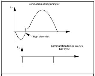
Fig. 7. Effects of rectifier-fed inductive load on phase control circuit
