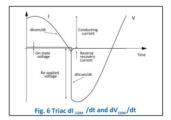
The dV<sub>COM</sub>/dt capability is affected by two conditions: -
