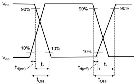
**Fig. 22. Switching time definition**
