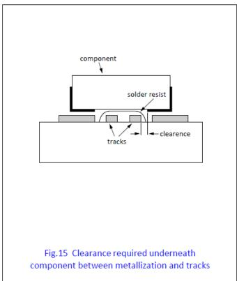
For components that need the additional clearance, the footprints on the following pages give the maximum space for tracks not connected to the solder lands (clearance  $\geq 0.1$ mm), for low-voltage applications. The number of tracks in this space is determined by the specified line resolution of the printed board.
