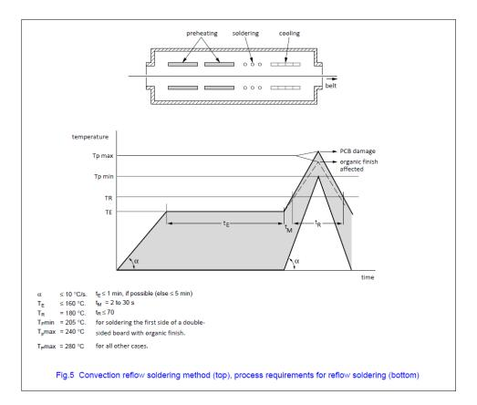
If soldering in a nitrogen atmosphere, a peak temperature of 280 °C is allowed for double-sided print boards or single-sided reflow soldering. Soldering in a nitrogen atmosphere results in smoother joint meniscus, smaller contact angles, and better wetting of the copper solder lands.
