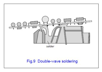
In principle, two different systems of PCB transports are available for wave soldering:
