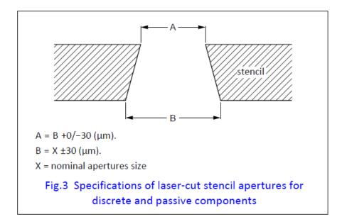
A useful method of controlling the stencil printing process during production is by monitoring the weight of solder paste on the board which may vary between 80% and 110% of the theoretical amount according to the target (designed) apertures. Smearing and clogging of a small aperture cannot be detected with this method.
