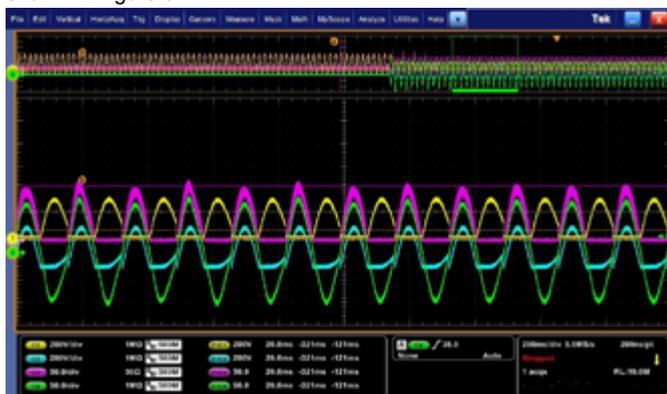
Figure 3: WeEn SCR: typical waveform used in UPS rectifier circuit (Purple: SCR1 A-K current; Yellow: SCR1 A-K voltage ; Green: AC mains current ; Blue: SCR2 A-K voltage)
