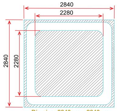
Die size: 2840μm x 2840μm Bond pad size: 2280μm x 2280μm
