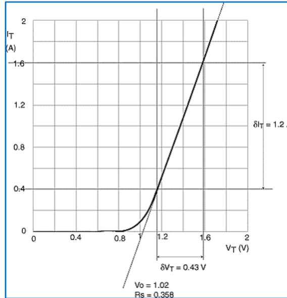
Fig. 25 Example graphic showing  $V_0$  and  $R_s$  derivation
