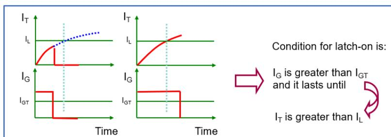
Fig. 21 Graphic showing interaction of  $I_{GT}$  and  $I_L$
