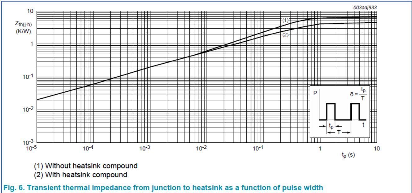
Fig. 19 Example of transient thermal impedance graphic
