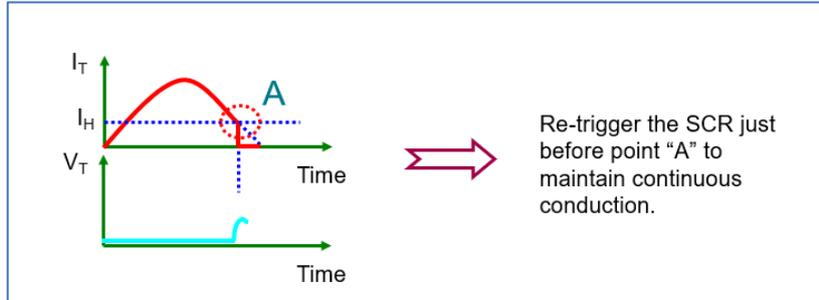
Fig. 22 Graphic showing interaction of  $I_T$  and  $I_H$
