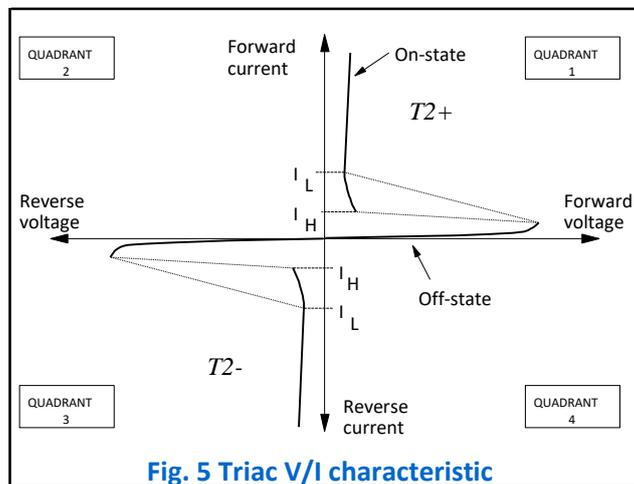
Where the gate is to be triggered by DC or unipolar pulses at zero-crossing of the load current, negative gate current is to be preferred. The internal construction of the triac means that the gate is more remote from the main current-carrying region when operating in the  $3^+$  quadrant. This results in: -
