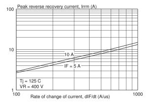
Fig.8. Typical peak reverse recovery current per diode,  $I_{rrm}$  as a function of rate of change of current  $dI_{e}/dt$ .
