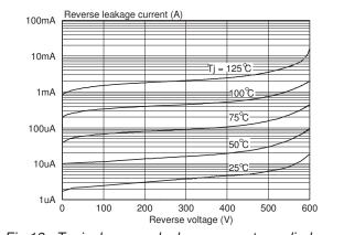
Fig.13. Typical reverse leakage current per diode as a function of reverse voltage.  $I_R = f(V_R)$ ; parameter  $T_i$
