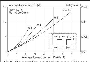
Fig.3. Maximum forward dissipation per diode as a function of average forward current; rectangular current waveform where  $I_{F(AV)} = I_{F(BMS)} \times \sqrt{D}$ .
