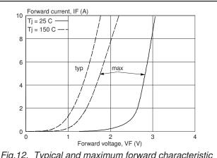
Fig.12. Typical and maximum forward characteristic per diode,  $I_F = f(V_F)$ ;  $T_i = 25^{\circ}C$  and  $150^{\circ}C$ .
