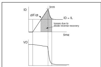
Fig.6. Origin of switching losses in transistor due to diode reverse recovery.
