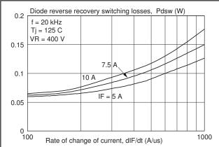
Fig.4. Typical reverse recovery switching losses per diode, as a function of rate of change of current dl<sub>F</sub>/dt.
