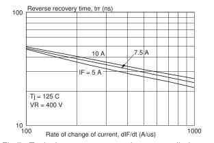
Fig.7. Typical reverse recovery time t<sub>rr</sub>, per diode as a function of rate of change of current dl<sub>r</sub>/dt.
