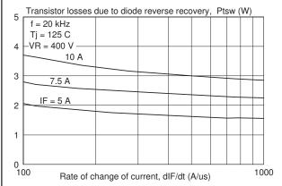
Fig.5. Typical switching losses in transistor due to reverse recovery of diode, as a function of of change of current dl<sub>p</sub>/dt.
