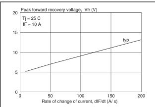
Fig.10. Typical forward recovery voltage per diode,  $V_{tt}$  as a function of rate of change of current  $dI_F/dt$ .
