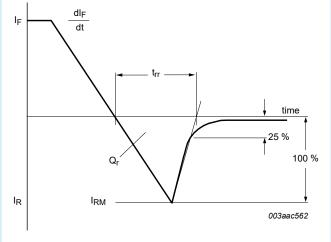
Fig. 7. Reverse recovery definitions; ramp recovery
