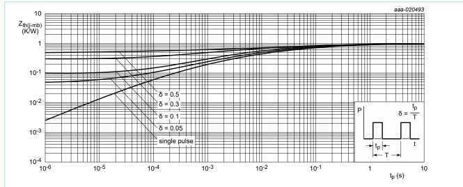
Fig. 5. Transient thermal impedance from junction to mounting base as a function of pulse duration; maximum values
