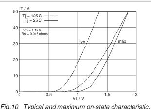
Fig. 10. Typical and maximum on-state characteristic.
