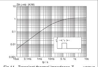
Fig.11. Transient thermal impedance  $Z_{th i-mb}$ , versus pulse width  $t_o$ .
